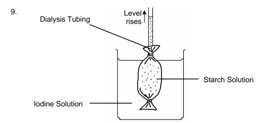
In the system illustrated above, a bag made from dialysis tubing (a semi-permeable membrane) is filled with a starch solution and immersed in an iodine solution in a beaker.
